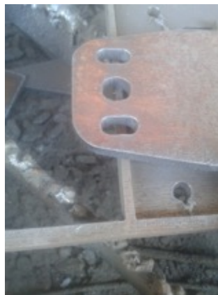
Improvements in hole and slot cut quality were observed in the part cut with genuine Cu+ consumables.
