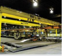
Overhead crane for moving raw materials and work-in-progress.
