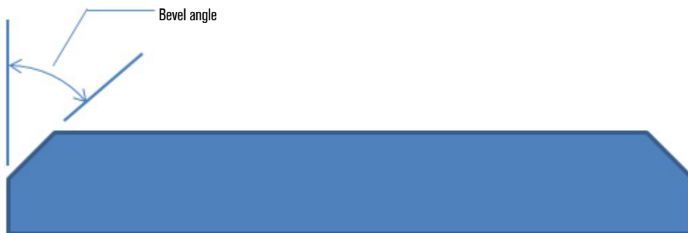
Figure 28 – Y Top cut bevel angle
