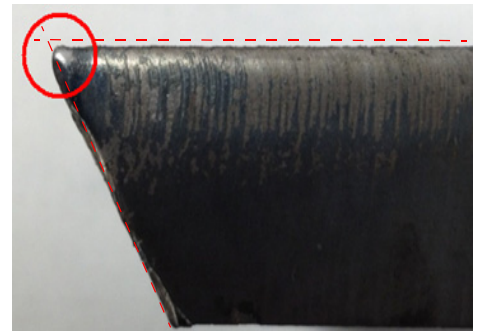
Figure 6 – A cut part size reduction due to top corner rounding
