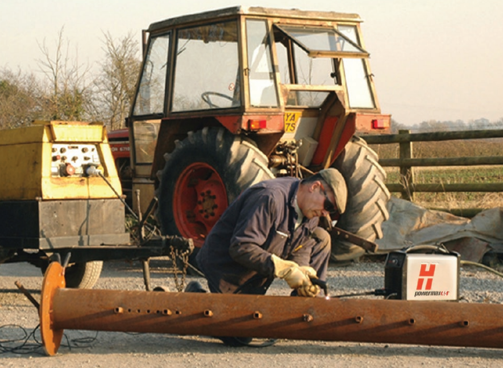
PLASMA BEING USED TO BACK-GOUGE FOR WELD PREPARATION IN A CUSTOM FABRICATION JOB ON A FARM.
