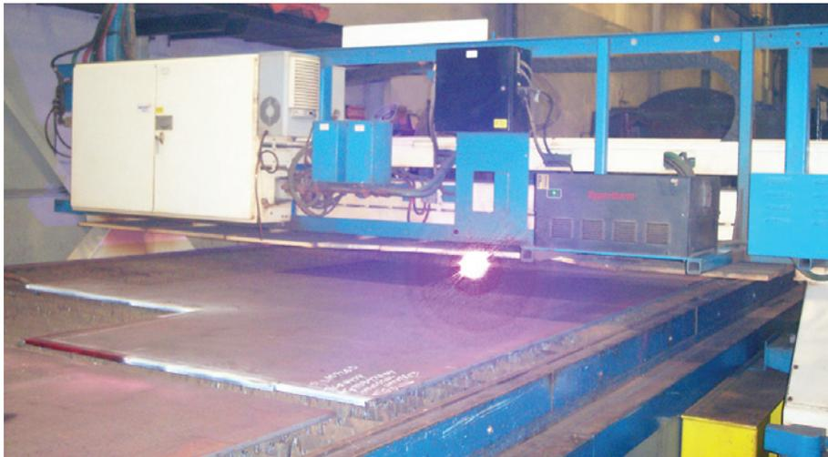
▲ The new high-definition plasma torches on Denman & Davis' plasma cutting machine allow it to reach tolerances of 0.003 to 0.004 inch.
