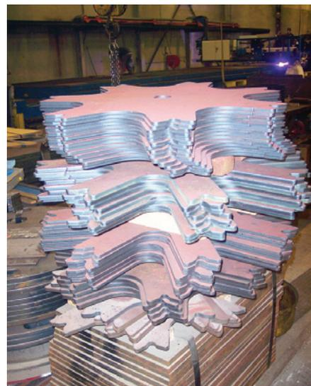
▲ Denman & Davis serves customers in industries as diverse as power generation and barge building. These plasma-cut gears are destined for a clothing-handling system designed for dry cleaning shops.
