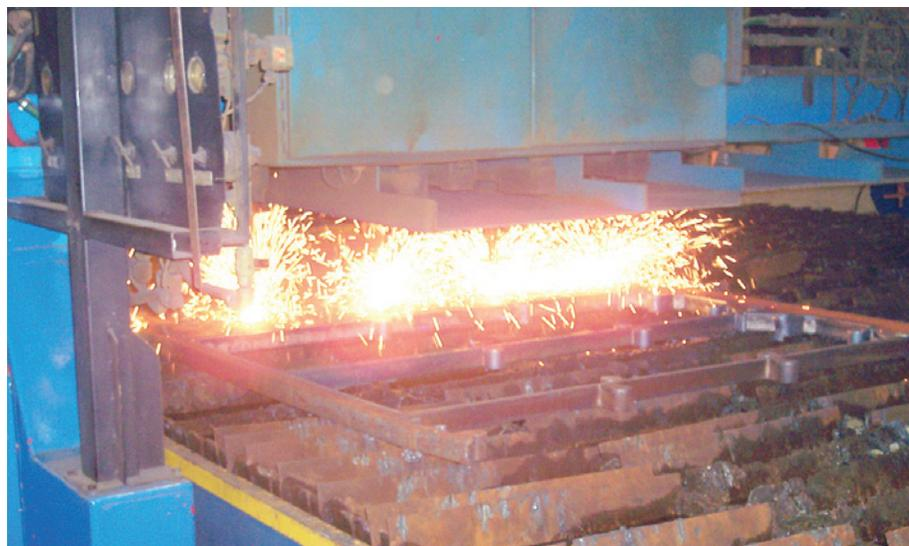
▲ Multiple cutting heads provide for a very efficient means of cutting plate.
