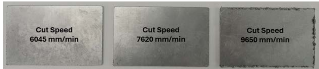
Figure 2 – Bottom view of three A380 samples cut at shown speeds using 85A air plasma with a 6.4 mm clearance height
