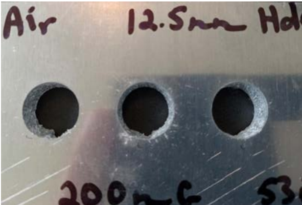
Figure 10 – 12.5 mm diameter plasma-cut holes in 6.4 mm thick 6061 Aluminum
