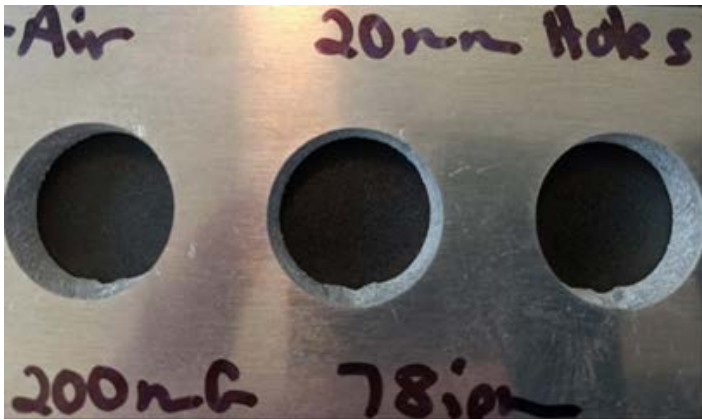
Figure 11 – 20 mm diameter plasma-cut holes in 6.4 mm thick 6061 Aluminum
