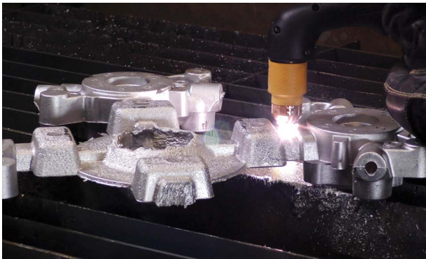
Figure 3 - Handheld plasma cutting
