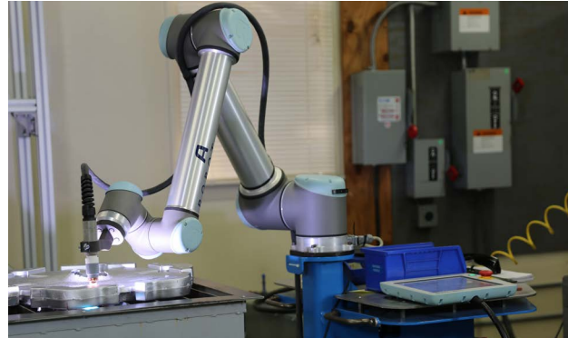
Figure 4 - Cobot plasma cutting
